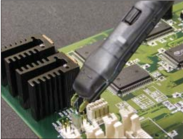
WaveLink high bandwidth differential probes let you capture head signals with best signal to noise ratio and low circuit loading.
